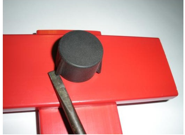
Nut Insulator (with ring) being prised off with the aid of a screwdriver.
