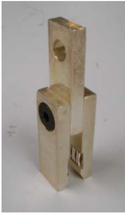
Contact for electrowinning cell. (approx 600A)
